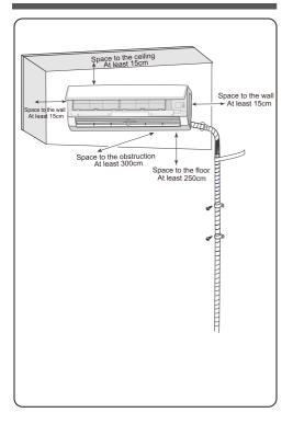
Safety precautions for installing and relocating the unit
