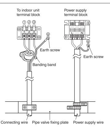
\* Clamp the indoor/outdoor connecting wire ③ and the earth wire together with the ferrite core with the supplied banding band. **Stripping length power cord and connecting wire**
