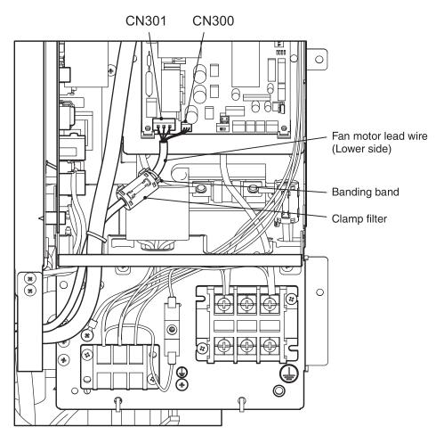
Attach the clamp filter supplied with the outdoor unit to the lower outdoor fan motor lead wire. • Make sure that the claw of the clamp filter is securely locked.
