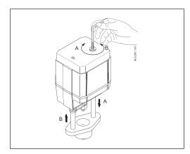
The manual override is applied by rotating the 4 mm Allen key (not supplied) to the required position. Observe the direction of the rotation symbol.
