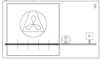
TT, S2 Pt1000 temperature sensor Р Pressure transmitter
