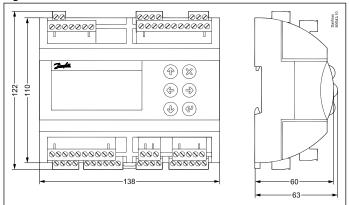
For DIN rail mounting only (IP 20)
