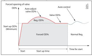
At start up. if the valve is opened too much, it could result in flow of liquid in the compressor or could trigger the HP switch which will stop the system. Whereas if you start the system with too low opening degree. it could also stop the system because of the low-pressure switch cut in. It will be safe to start the system with approximately 50% OD of the valve at start up, if P-control is not being used.
