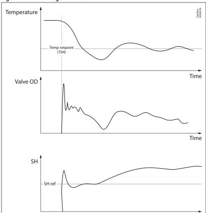
Figure 10: Modulating thermostat
