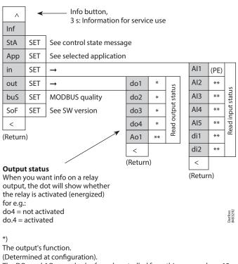
The DOs and AOs can also be forced controlled from this menu, when r12 Main switch has been set in position "service".
