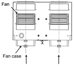
Align center of the fan with that of the fan case.
