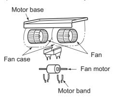
Note: After the fan has been replaced, pay attention to two followings to assemble each component. 1. After the fan was fixed, check that it turns smoothly without coming in contact with a fan case when turned by hand.
