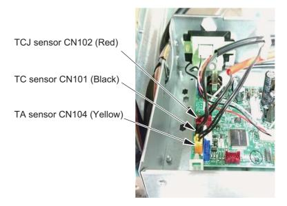
Position of Relay connectors for remote controller
